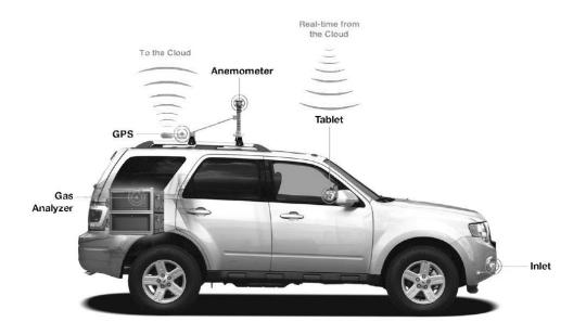
While less than \$100,000, the Picarro AMLD also included the purchase of a vehicle under work order 0042W0007758, which was inter-district transferred to Southern Nevada where the Picarro AMLD is installed and operated. In addition to leak patrols, the Company uses Picarro AMLD to collect methane plume data which is routed to back-end data analytics software.
